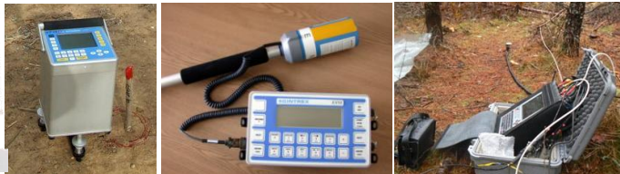
Grawimetry CG-5/CG-SHT, SCINTREX Ltd.; magnetometry ENVI PRO, ENVI TOTAL FIELD, ENVI-GRAD-VLF SCINTREX Ltd.; System 2000.net, PHOENIX-GEOPHYSICS Ltd.
