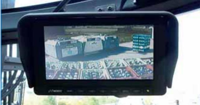
Typical configuration view over the load / rear area surveillance
