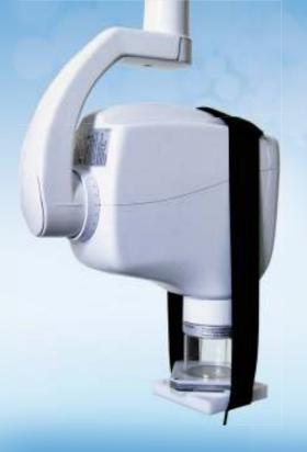
The Pro-Dent set is a **universal set of phantoms** for carrying out constancy and acceptance tests of **conventional and digital** dental X-ray units (intra-oral, panoramic and cephalometric). This is not an all-in-one device where results of tests blur each other out. This is the only solution on the market that allows measuring of the x-ray beam radius at the end of the beam applicator.
